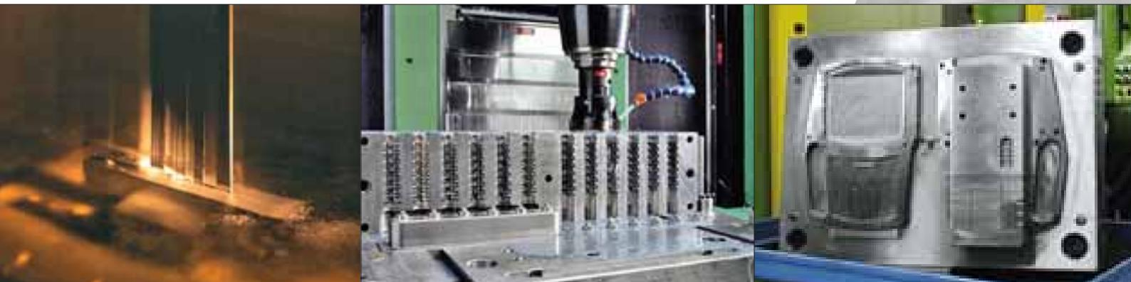
*3d CAD files of the mold parts created in our technical office, are sent via computer network to our shop, that makes every single mold component out of **top quality steels**.*
